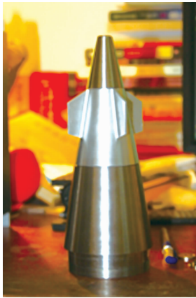
图 12 可控滚转修正机构 Fig. 12 Spin controlled trajectory correction mechanism
