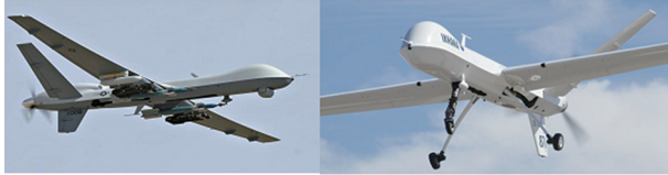
图 2 捕食者无人机操控面布局及起落架装置 Fig. 2 Control surface layout and landing gear of Predator UAV
