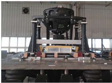
图6 重力梯度仪垂向振动试验现场图 Fig.6 Field diagram of vertical vibration test for gravity gradiometer
