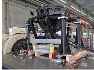
图8 重力梯度仪水平振动试验现场图 Fig.8 Field diagram of horizontal vibration test for gravity gradiometer
